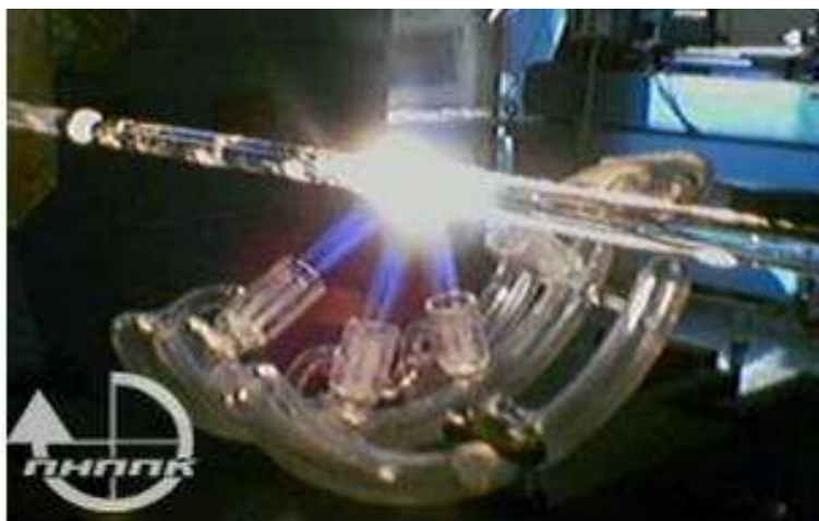
Fig. 11. Four-sectioned quartz burner and preform in MCVD
